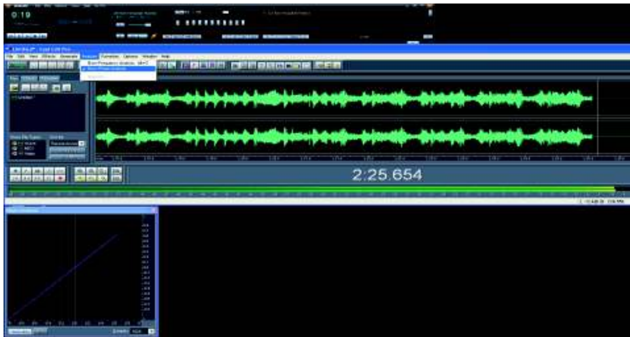
A mono signal will have a bar at 45 degrees upwards from left to right.
